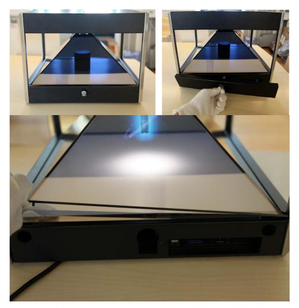
With a finger through one of the holes, it is now possible to lift the piece of optic facing the door. Lift the optic slightly and pull it gently downwards until it comes loose from the metal lamp house in the top. There is no need to release the optic from the metal spring holding it, unless you wish to replace the optic with a new one.
