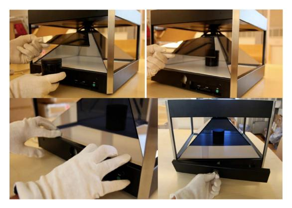
**NOTE**: When the object has been placed in the chamber and the optic should be set back in place, it is important to make sure the top of the optic is positioned in the right place. It should, without the use of force, slide up in the space at the top of the pyramid, where the four optics meet, and gently be pushed into the right position.
